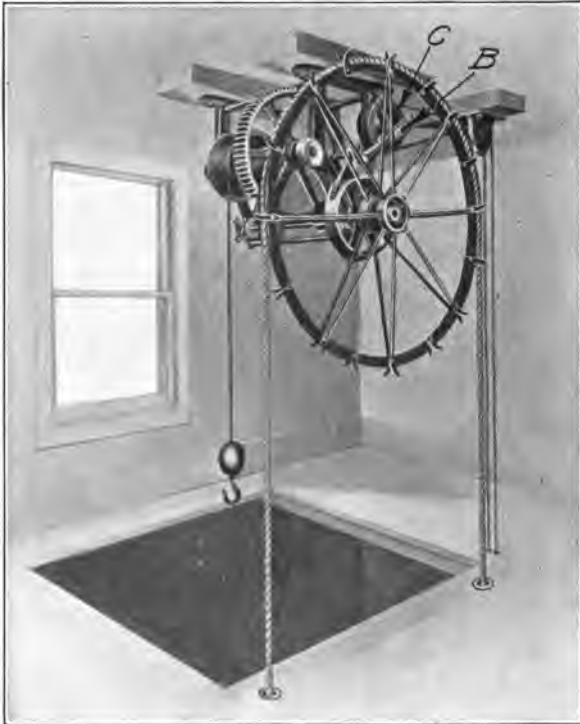
Fig. 16. Rope Hoist with Band Brake but without Ratchet and Locker Courtesy of Warsaw Elevator Company, Warsaw, New York
